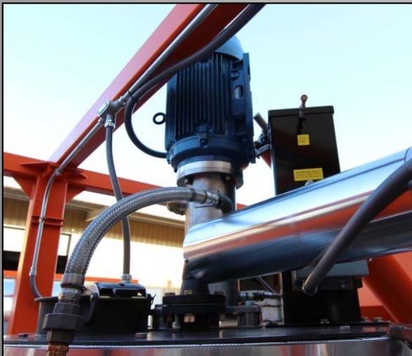
High speed / high shear mixer unit with watered cooled bearings
