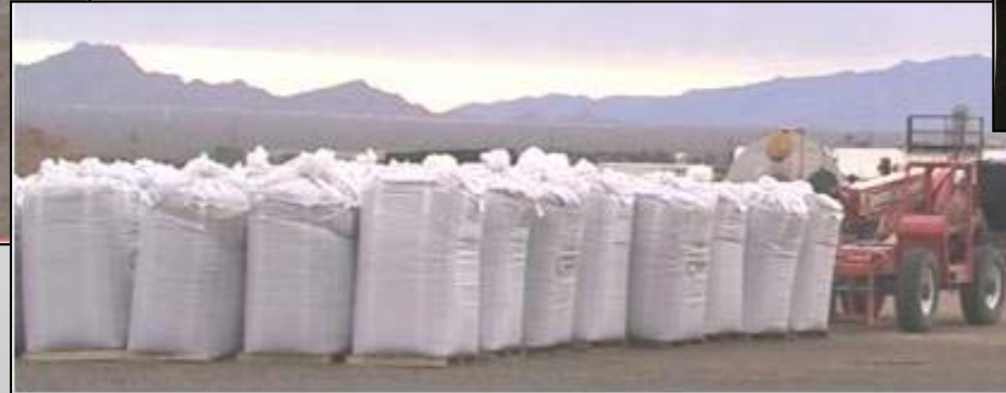
Crumb Rubber Is Delivered To Site In One Ton Super Sacks (approx. 1,000 Kilos each)
