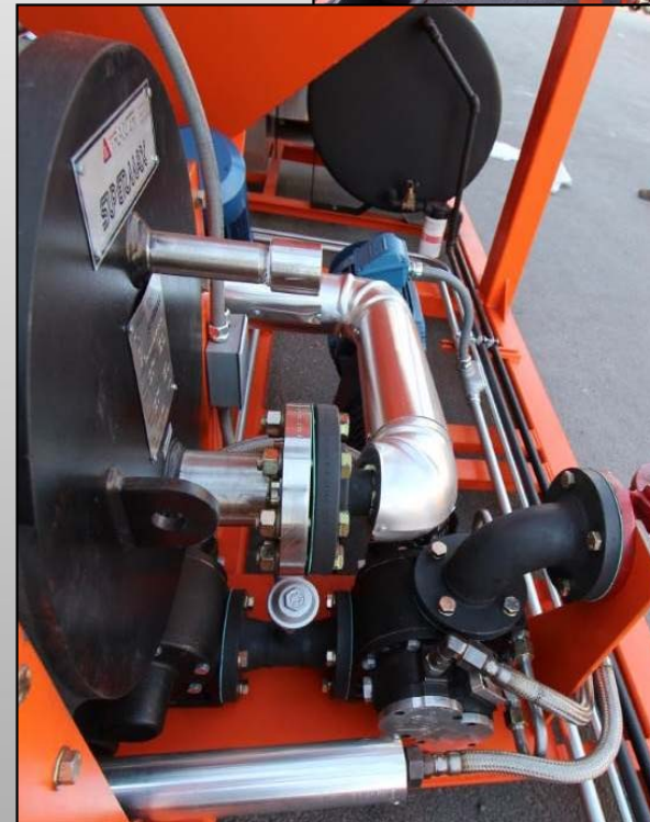
Heat exchanger to raise the temperature of the incoming bitumen before adding the crumb rubber
